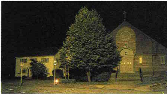
Under the light from high pressure sodium lamps, the white house, green tree, and brown church at this site all blend to a yellow hue. (PHOTO: GARY CLAYTON HALL)
