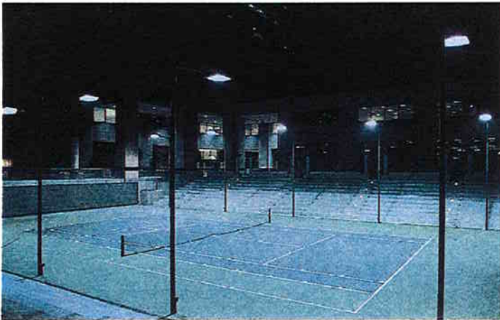
Sports facilities can be adequately lit using non-glare cut-off fixtures.
