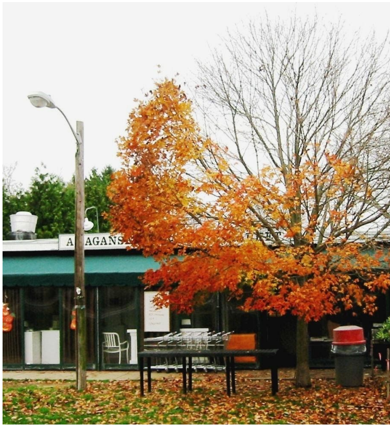
Sag Lens cobrahead directs light upward. Leaves “fooled” into hanging on into dormancy.
